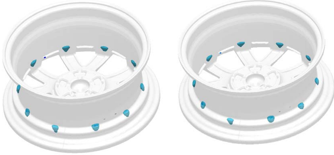
Figure 8. Comparison of the analysis porosity results with old and new casting setup cards (the old setup on the left, the new casting setup result on the right)
